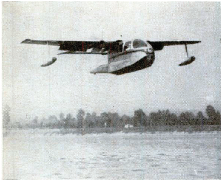
Above: After a 1,500-foot run the Riviera is airborne from a lake. Aircraft was originally designed by Fiat-Nardi and still bears designation FN-333. The SIAI-Marchetti firm then acquired license to build the amphibian in 1959.
