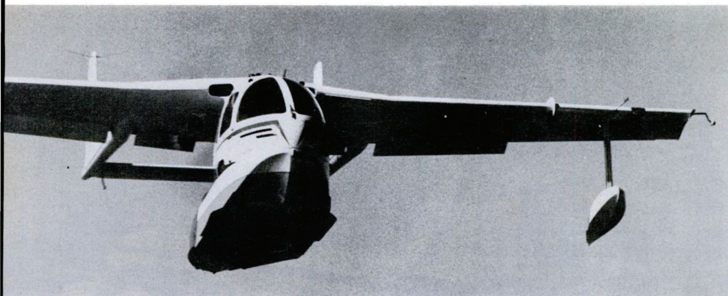
Aerodynamic fences two thirds of the wing length out from the center section enhance low airspeed characteristics. Maximum speed is set at 177 mph.
