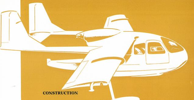
All parts of the aircraft which are immersed in water or may make contact with it, have been made of nickel alloy and stainless steel.
