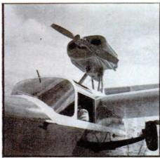
ing the three-point attitude, you'll notice the Teal's rather shallow pitch position. The designers didn't want to make the main gear longer than necessary; the result is that it's a bit shorter than ideal for full-stall landings. Citabria pilots will recognize the probable effect of this characteristic: occasional tailwheel-first landings, with the main gear plunking down a fraction of a second later.
