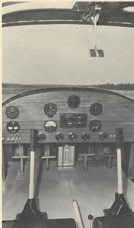
Sport flyers will delight in the stick control but instructors will have to have dual brakes not shown on this model. Throttle lever is mounted overhead in seaplane fashion. It is understood that shoulder harness will be incorporated in production aircraft providing good cockpit safety.
