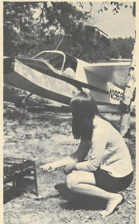
Conventional landing gear makes beaching in muddy or rough beach area easy and spring steel landing gear can take its lumps without problems.
