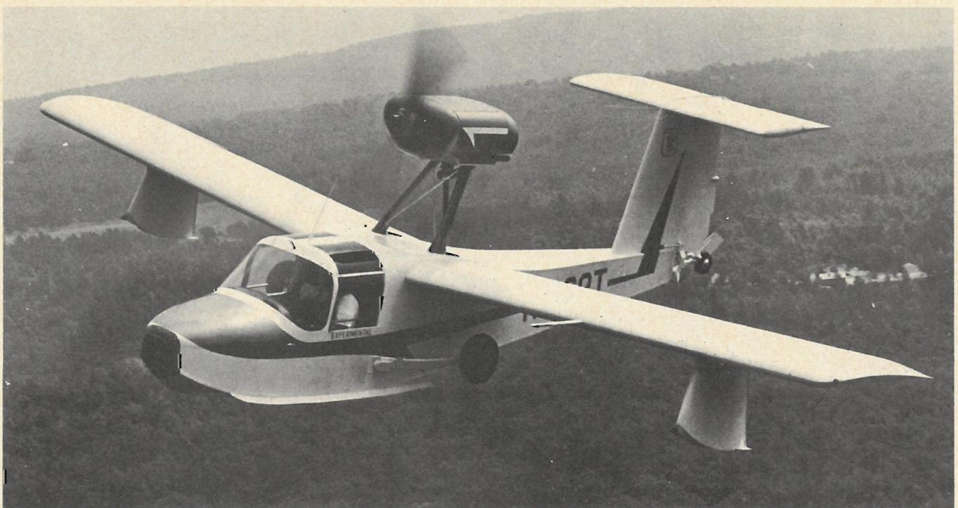
For the first time in many years, land locked operator can offer seaplane training with this outstanding little amphib tractor. 22 Engine pod offers quick servicing of power plant.
